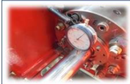
Piston rod drop inspection
