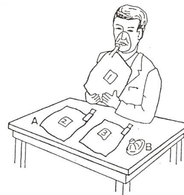
Fig. 18 Method of sniffing in triangle odor bag method
